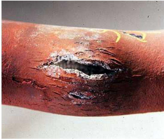
Photo 160-a1-5 Over-heating due to deposit
