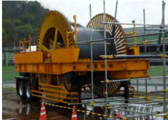
Figure 70 Transport cable drums
