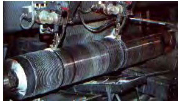
Photo- 14: Hard-facing welding of roller
