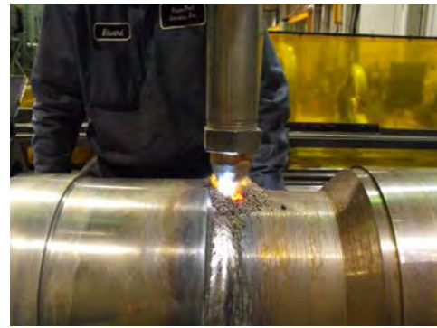
Photo- 20: Submerged arc welding of GT rotor
