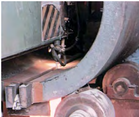
Photo- 3: Longitudinal welding of thick part
