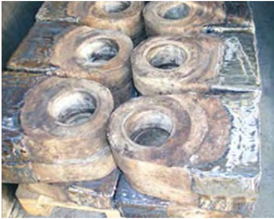
Photo- 11: Crusher hammers after repair
