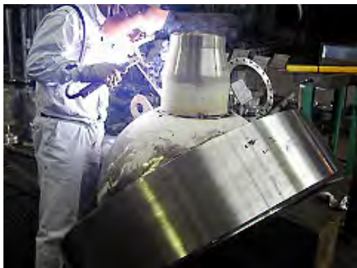
Photo- 5: Welding of thick parts
