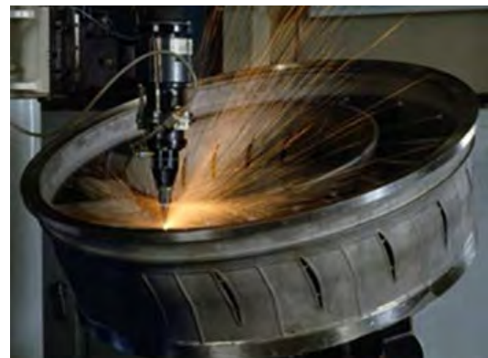
Photo- 10: Laser beam welding of GT swirler
