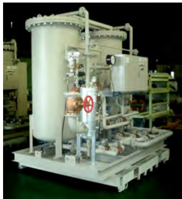
Photo- 5: Pressure swing absorption equipment
