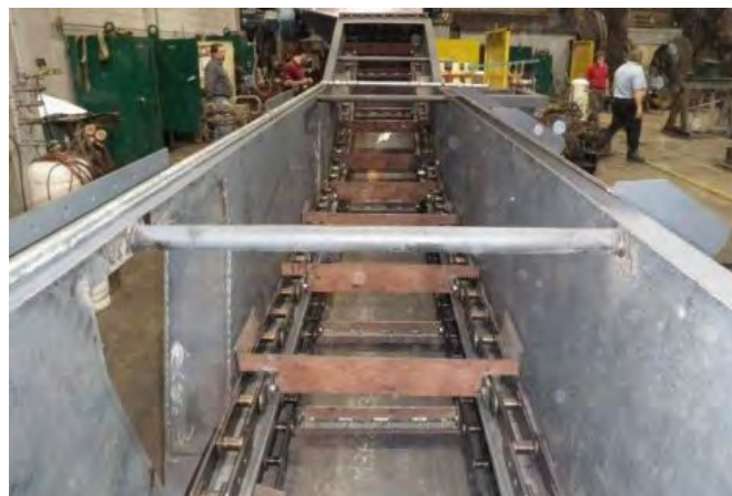
Photo- 13: Water seal chain conveyor
