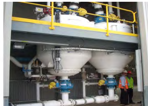
Photo- 6: Dence phase pneumatic transporter
