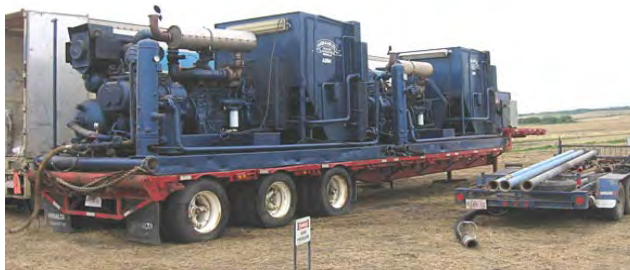
Photo- 27: Compressor for pressure test
