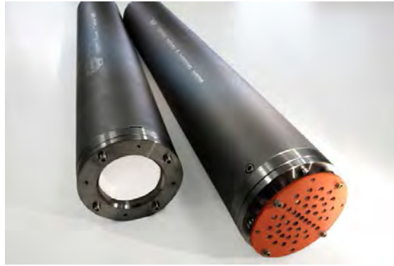
Photo- 37: Hydrocarbon & methane sensor
