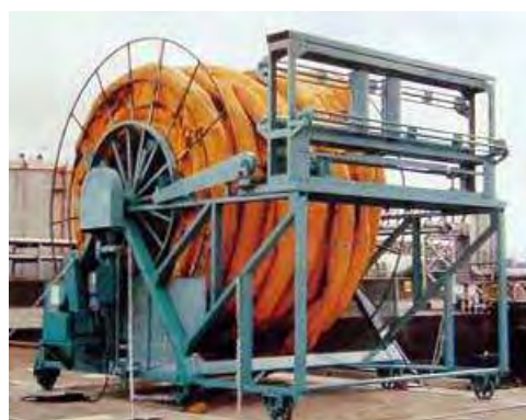
Photo- 124: Oil fence
