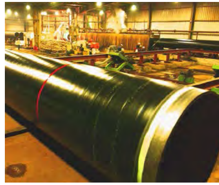
Photo- 57: Fusion bonded epoxy powder coating
