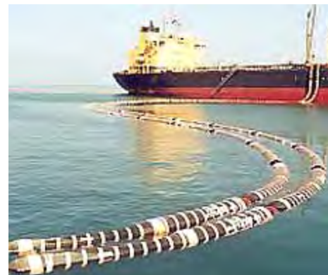
Photo- 18: Marine hose for unloading
