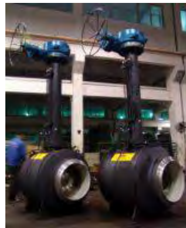
Photo- 95: Stem extension valve for underground pipeline
