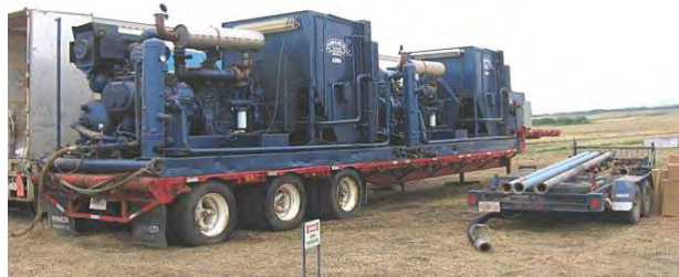
Photo- 87: Compressor for pressure test
