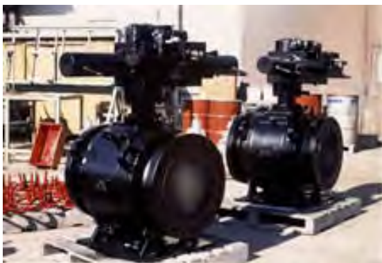
Photo- 29: Shut-off valve between marine hose and subsea pipeline
