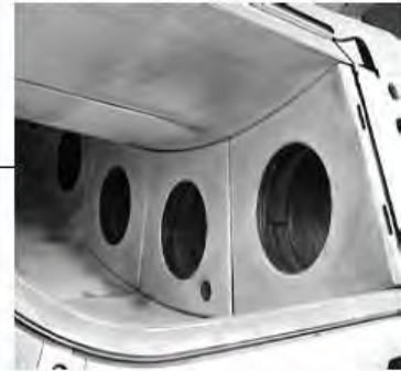
Annular Combustor in GT8C2, GT13E2, GT24 and GT26
