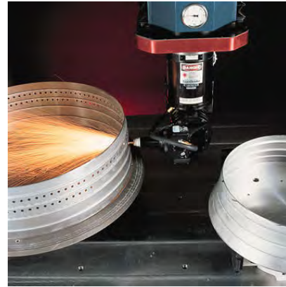
Photo- 45: Laser drilling of combustor
