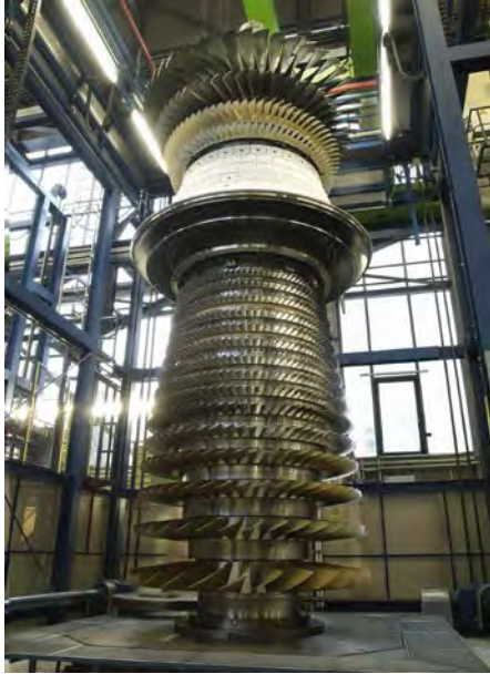
Photo- 47: Gas turbine rotor assembly
