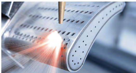
Photo- 59: Laser drilling of GT blade
