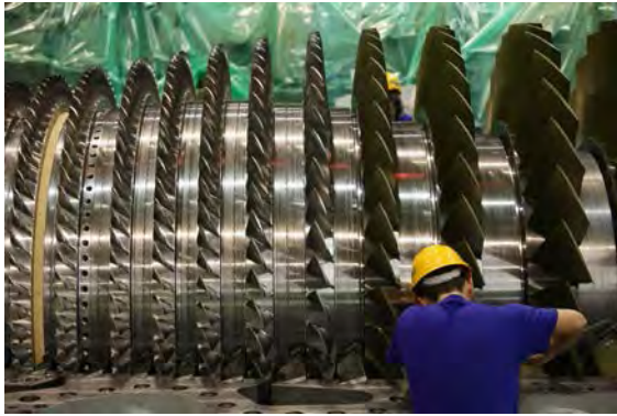
Photo- 71: Compressor blade
