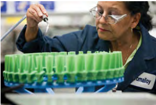
Photo- 58: Lost wax casting of blade
