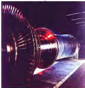
Maintenance free, welded rotor in all ALSTOM heavy duty gas turbines
