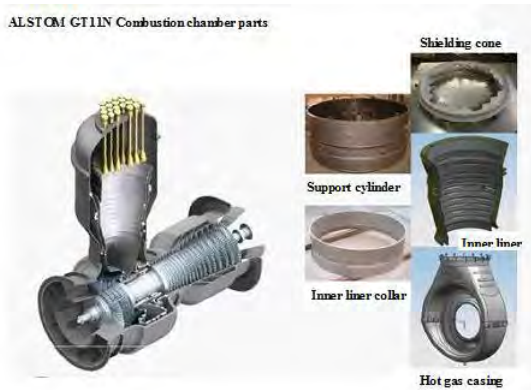
Photo- 46: Silo type combustor
