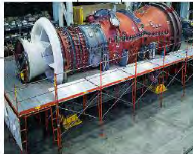
Annular Combustor in GT8C2, GT13E2, GT24 and GT26
