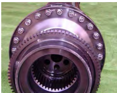
Photo- 35: Coupling with spline for a solar gas turbine application
