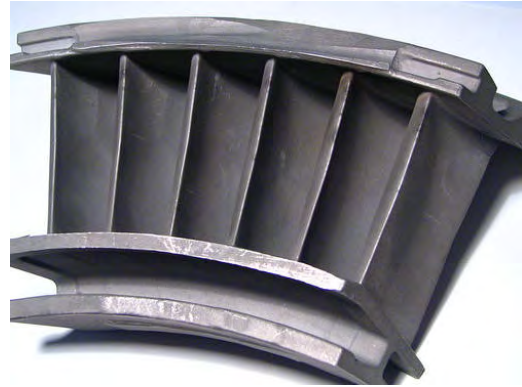
Photo- 61: Gas turbine vane segment
