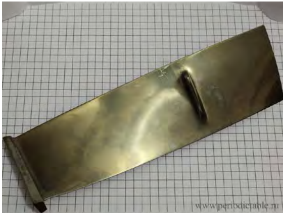
Photo- 67: Compressor blade
