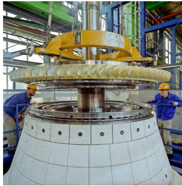
Photo- 48: Assembling of gas turbine disc
