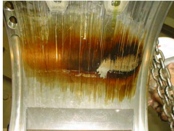
Photo- 32: Varnish formation on GT bearing http://www.realservices.com/Spotlight/Ferrogaphy-Power-Plant.htm
