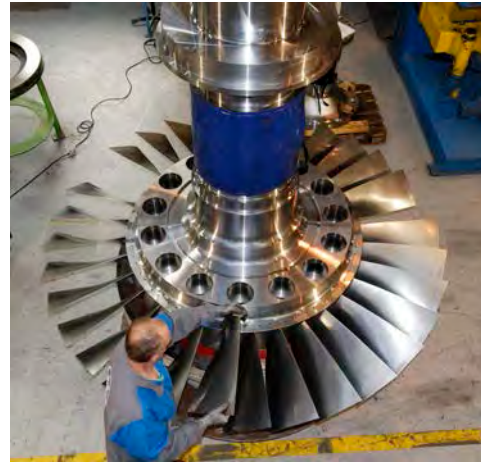
Photo- 52: Compressor rotor head
