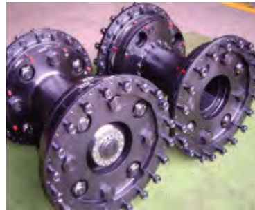
Photo- 34: Load Couplings with shear pin arrangement for gas turbines rated 16 MW at 1500 rpm
