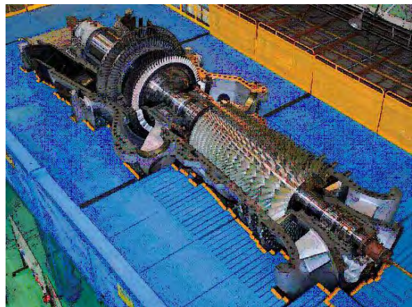
Photo- 6: 90MW class GT (Hitachi-H80)
