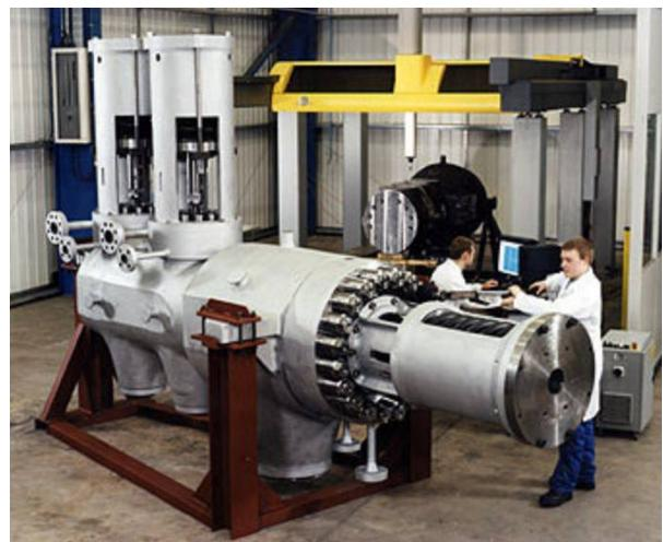
Photo- 33: 600MW class main stop valve
