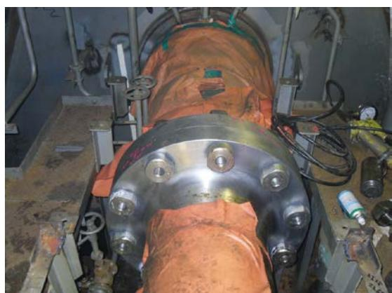
**Photo- 20: Coupling and coupling bolt**
