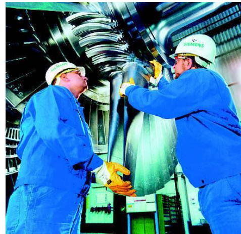
Photo- 24: LP turbine blade (Siemens)
