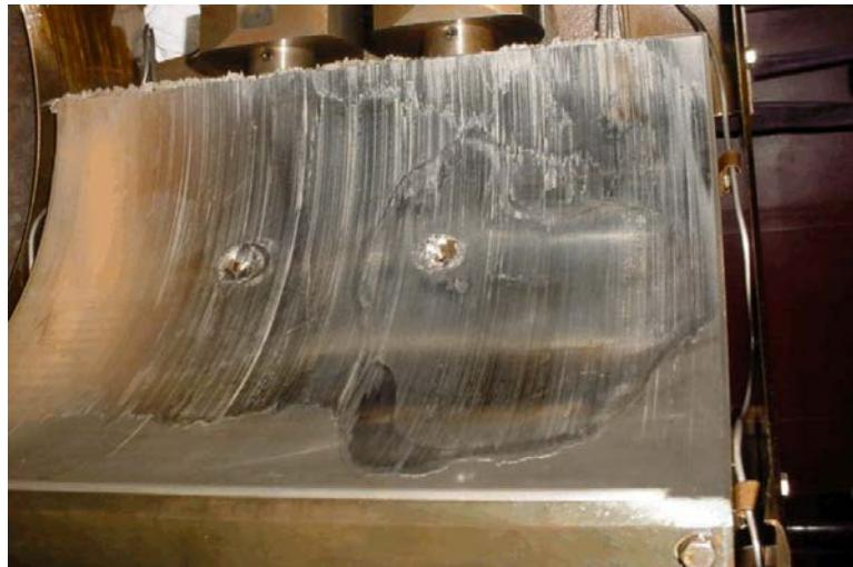
Photo- 27: HP bearing quickly destroyed by shaft current
