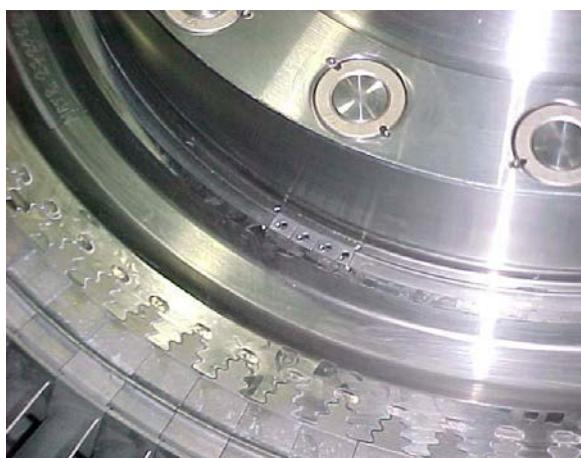
Photo- 30: Installation of balancing weight
