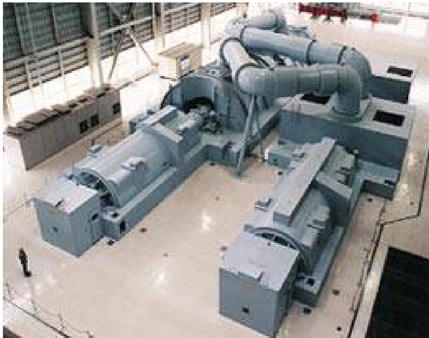
Photo- 8: Typical construction of steam turbine (cross compound type 1,000MW class)
