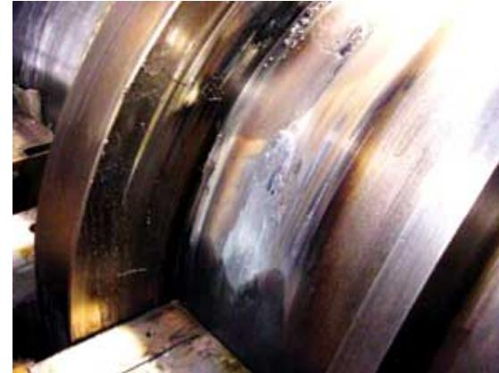
Photo- 14: Damaged thrust bearing
