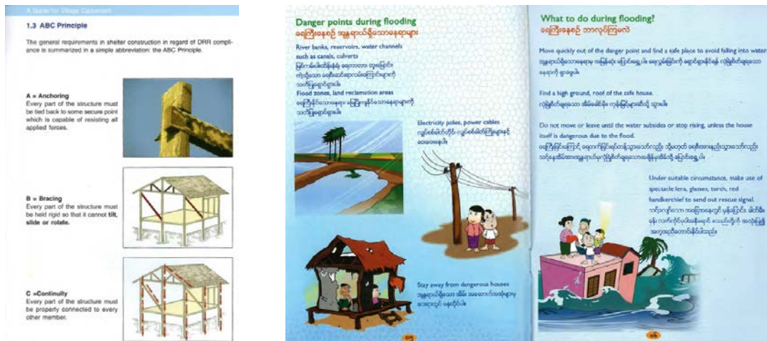
a) Guidance How to Construct Safe House
