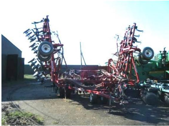
Picture 7-1: combined machine of large grain drill, cultivator and roller
