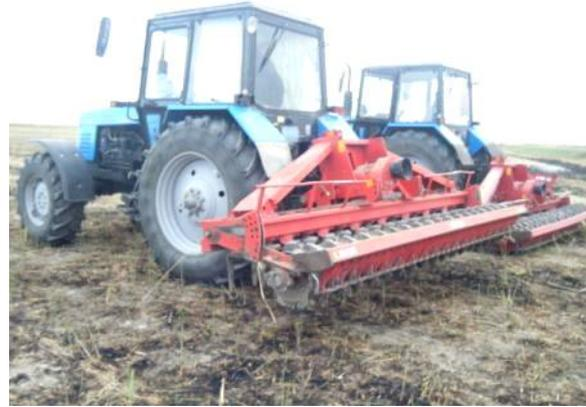
Picture 7-2: combined machine of rotary and suppresser
