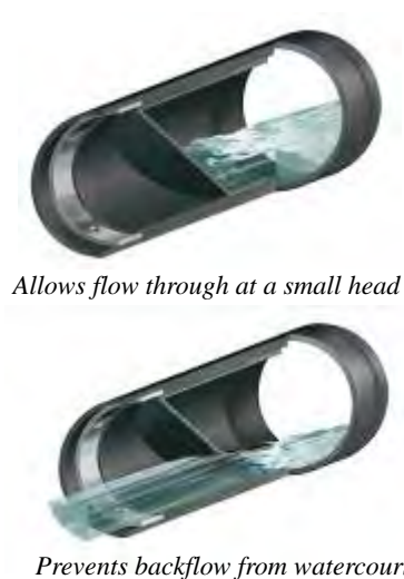
Figure 5.11.13 Inline Check Valve
