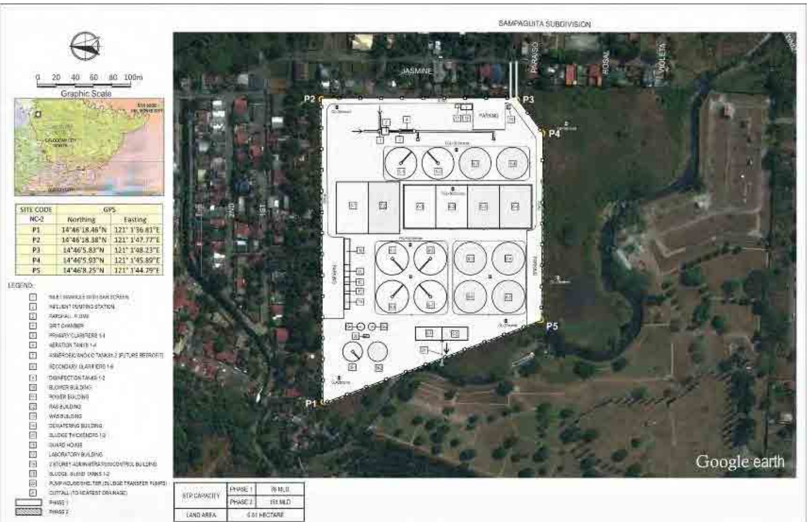
Source: IICA Study Team Figure 5.3.10 Facility Layout of STP in the Marilao River Basin (Option 2)
