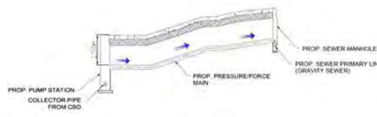
Figure 5.1.8 Pressure Main Profile
