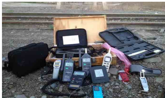
Figure 57. Tools used for measuring of noise level nearby proposed Flyover bridge
