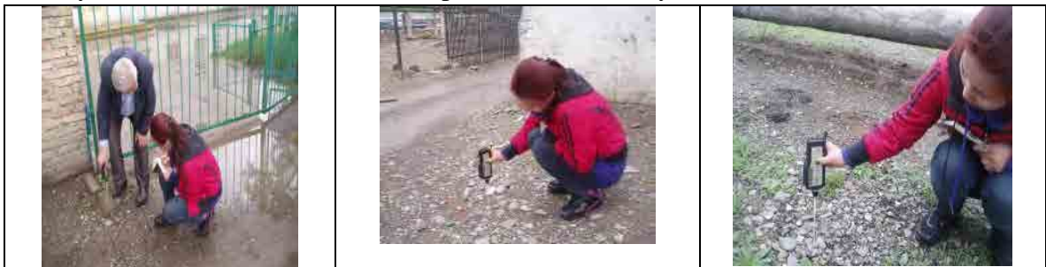
Figure 61. Vibration was measured by a sensor at the surface level, where vibration is coming
