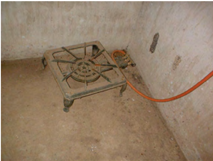
Figure 4.5.7: The Biogas Stove that is meant to replace traditional charcoal/firewood stove
