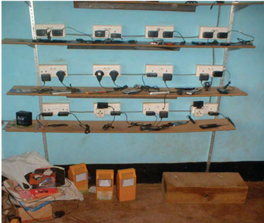
Figure 4.2.6: Charging station. The LED lamps (Accendo from India, yellow ) seen on the ground
