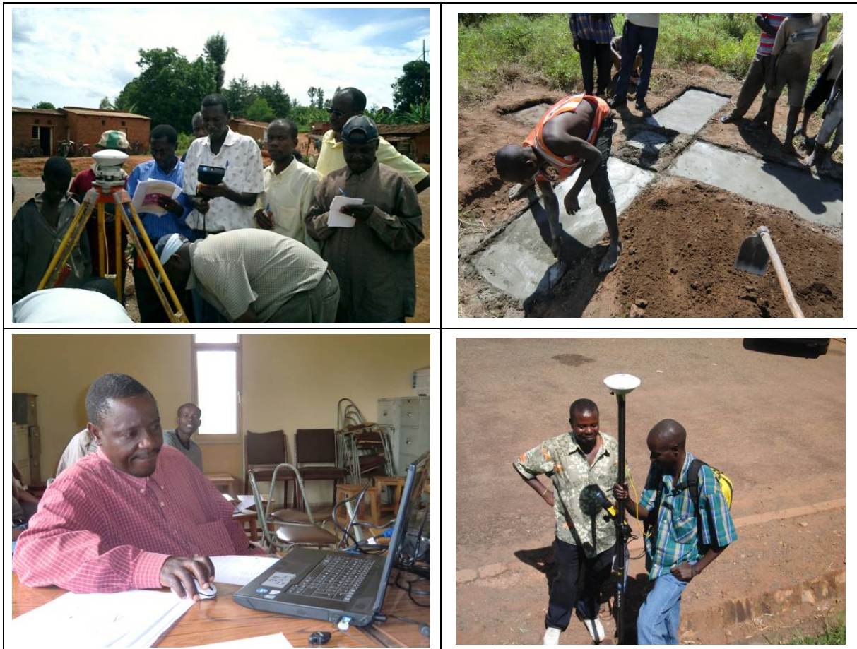
Figure. 39 Scenes in the Technology Transfer on the Ground Control Point Survey (Upper left: GPS observation, upper right: installation of a pre-mark, lower left: network adjustment, lower right: application of the GPS observation)
