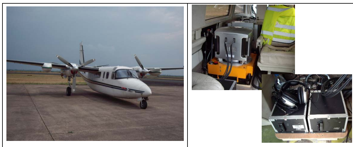
Figure. 11 Photographing Equipment (Left: aircraft used for photography, right: digital camera, GPS/IMU)
