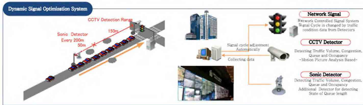
Expansion of Adaptive Signal Control
