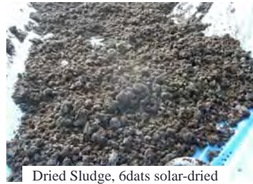
Dried Sludge, 6 days solar-dried
