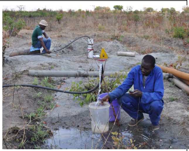
6. Constant discharge test at TTC No. 3
