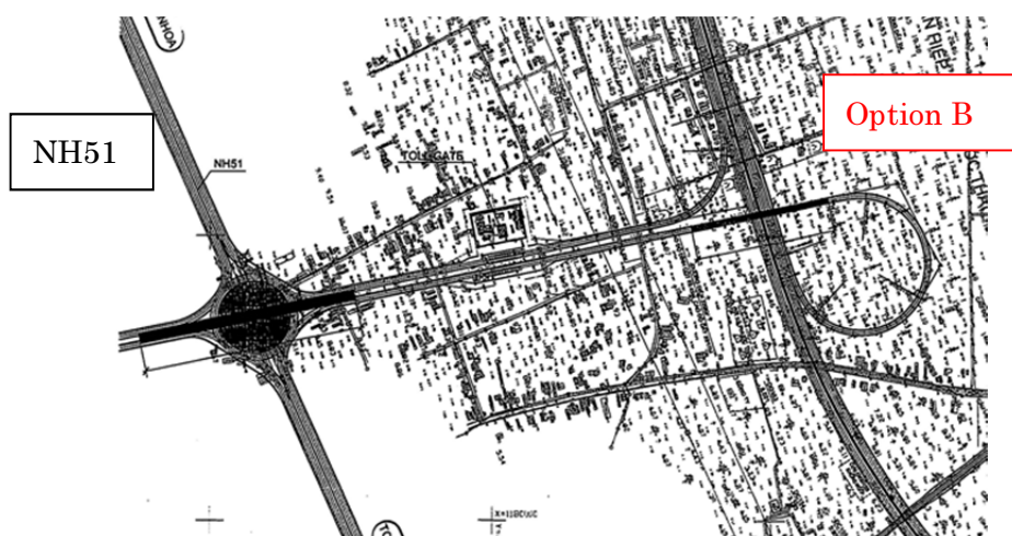
Figure 5.2.16-7 Layout of Partial Trumpet Type
