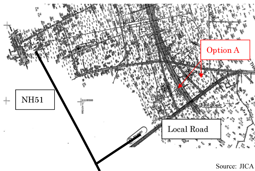
Figure 5.2.16-6 Layout of Half Diamond Type
