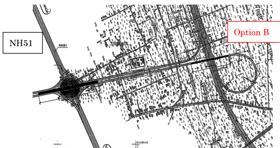
Figure 5.2.16-7 Layout of Partial Trumpet Type
