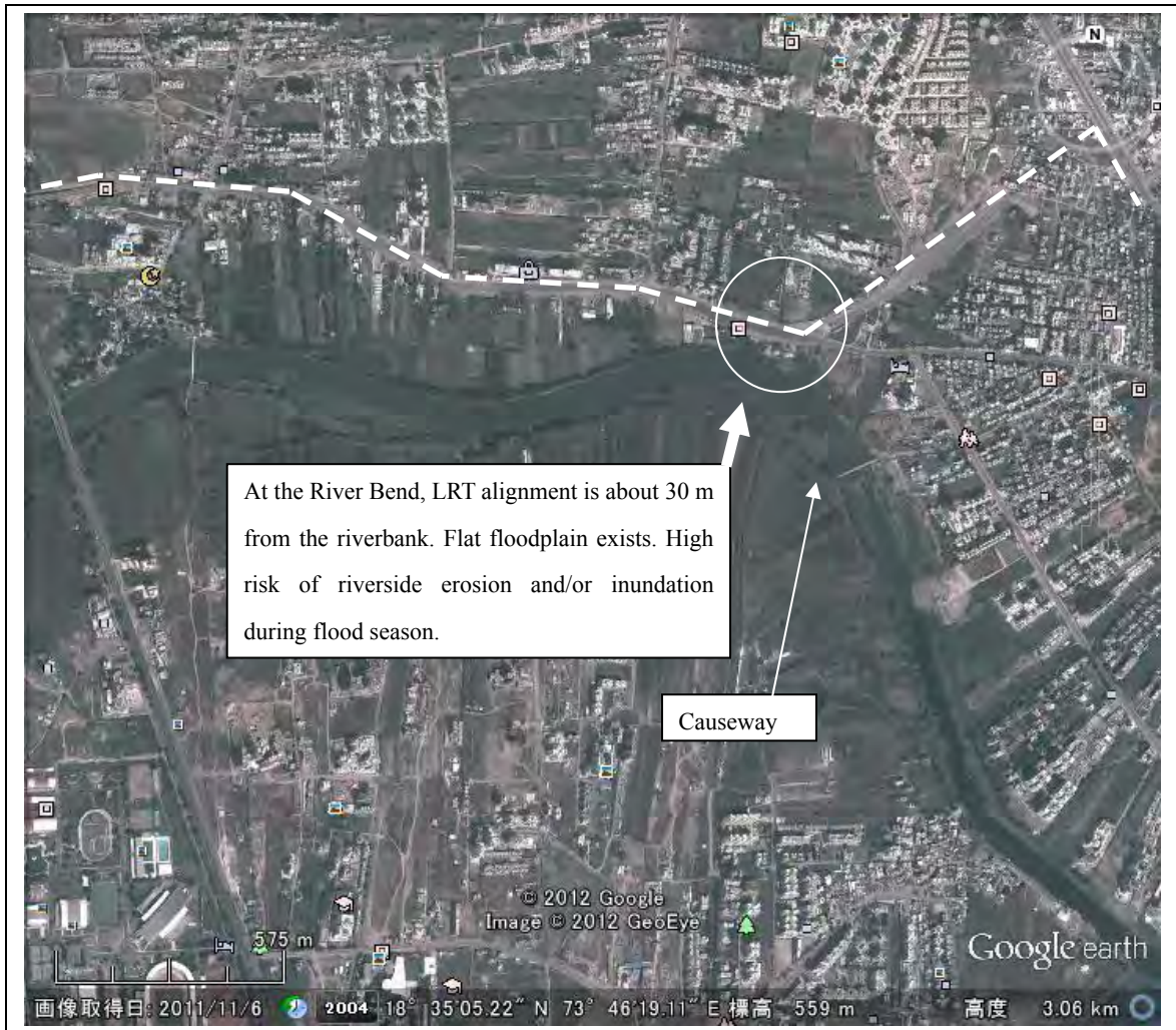
Figure 7.5.5 Mula River and LRT Alignment
