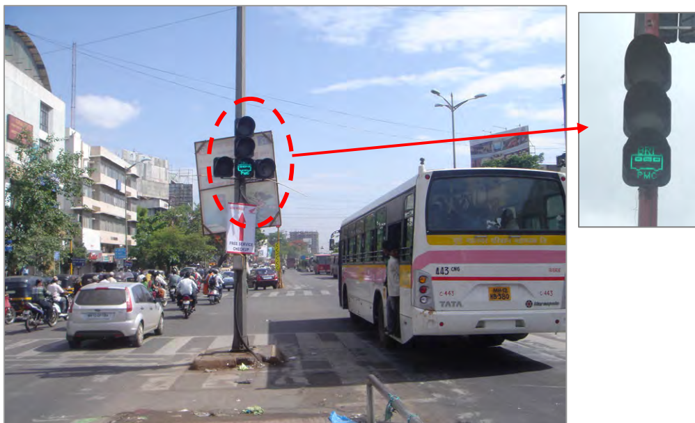
Figure 5.5.9 BRT Priority Signals along BRT Route in PMC
