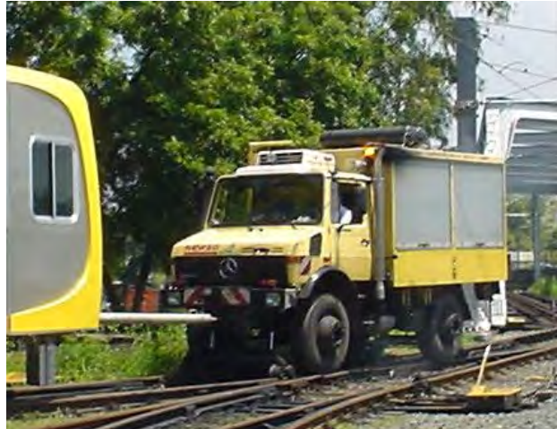
Figure 5.4.18 Sample of Road Rail Vehicle (Manila LRT Line 1)
