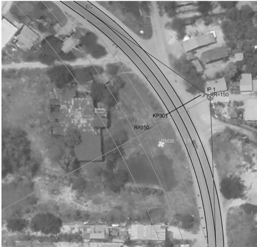
Figure 10.2-5 New Alignment at IP1
