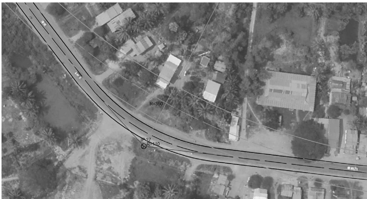
Figure 10.2-7 New Alignment at IP27 (KP 355 + 485)
