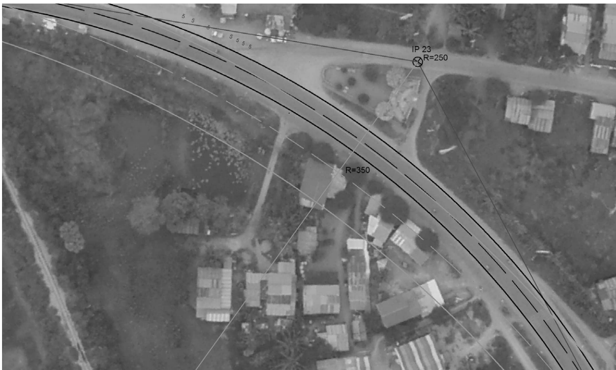
Figure 10.2-6 New Alignment at IP23 (KP 351 + 797)
