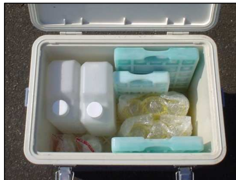
Photo: Sample Transportation with Refrigerant or Ice
