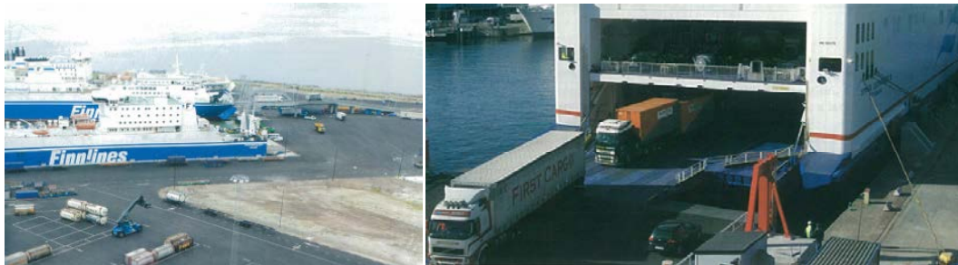
A RO-RO ship with stern ramp and/or bow ramp – this type RO-RO ships usually dock at L-shape berth where a shore ramp is equipped – car deck space of a RO-RO ship will be fully utilized to accommodate vehicles or cargoes in comparison with a RO-RO ship with quarter ramps – small ships is likely to be this type
