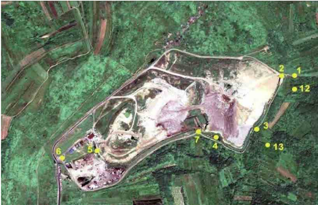
Figure 28. Water sampling locations at the Vinca landfill site perimeter (Source: Local Waste Management Plan for the City of Belgrade 2011-2020, 2011)
