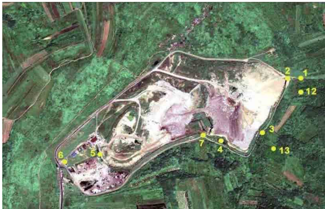
Figure 31. Water sampling locations at the Vinca landfill site perimeter (Source: Local Waste Management Plan for the City of Belgrade 2011-2020, 2011)
