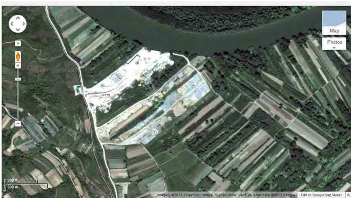
Figure 14. An aerial shot of the location of the WWTP. The silver areas are the interceptor building plateau and the silver/ brown/ blue areas are deposits of excavated materials from the interceptor tunnel.
