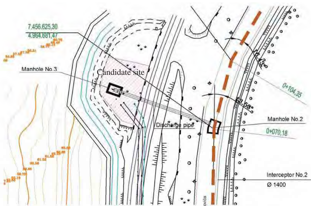
Figure 4.11 Candidate Site for Departure Shaft of Drainage pipe
