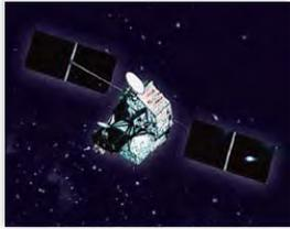
TRMM is an Earth-observation satellite that diagnoses conditions on Earth by measuring precipitation in tropical and subtropical areas.
