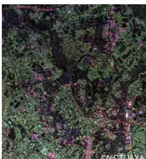
Strong back scattering in urban area from buildings inside. Reflection from building face to wave incidence causes strongest back scattering.
