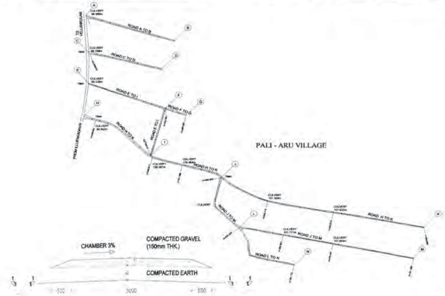
TYPICAL DESIGN SECTION -ROAD 3.0m
