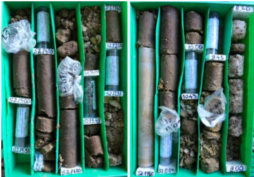
Figure 4 – Samples recovered from borehole S1 (above) and S2 (below)
