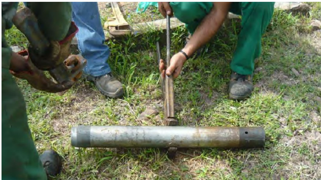
Figure 8 – Moran sampler used for undisturbed sampling
