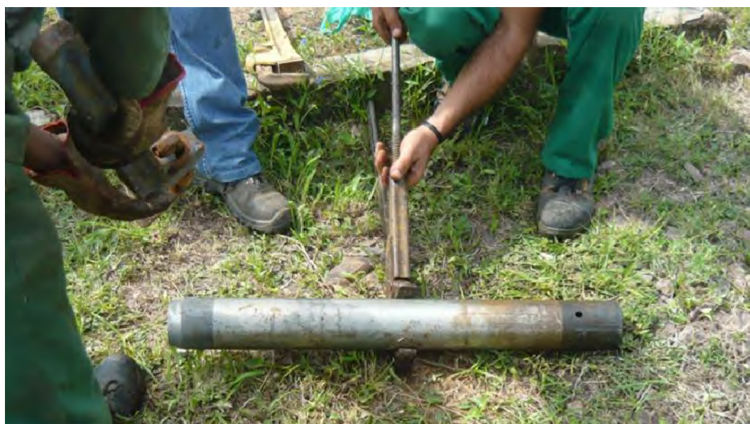
Figure 8 – Moran sampler used for undisturbed sampling
