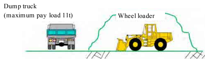
Figure 7-7 Loading and Transportation
