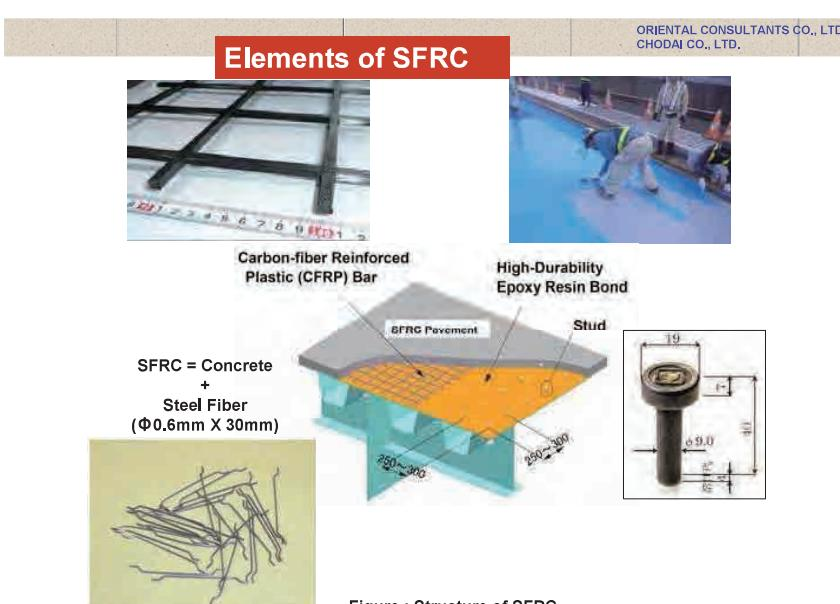
Figure : Structure of SFRC
