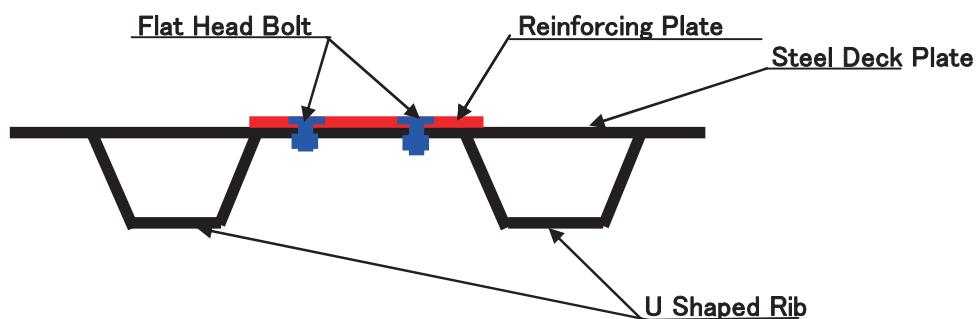
**Figure 1 Reinforcing Plate of the Steel Deck Plate**
