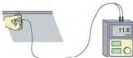
**Figure C.3 Plate Thickness Inspection by Ultrasonic Inspection**
