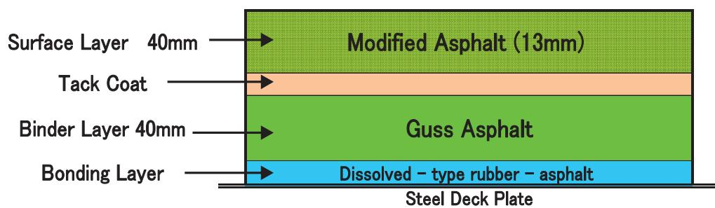
Figure –1 Pavement Structure of Guss Asphalt Method
