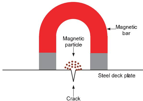
**Figure C.1 Magnetic Particle Inspection**
