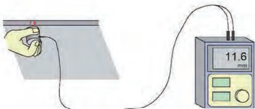
Figure C.3 Plate Thickness Inspection by Ultrasonic Inspection
