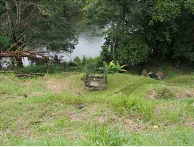
Piezometer installed at the lower part of the landslide.
