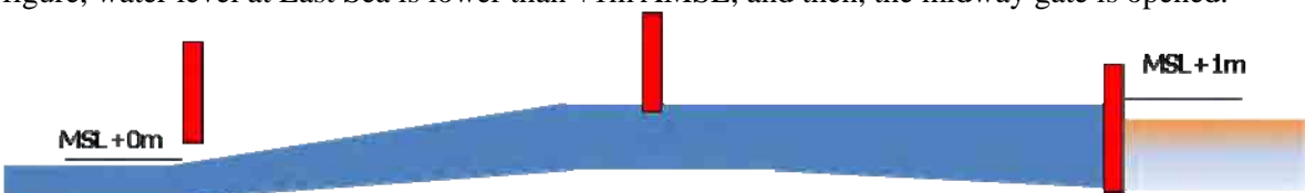
Figure 3.6.3 Gate Operation; West Sea water level is lower than 0m AMSL, the West Sea Gate is opened
