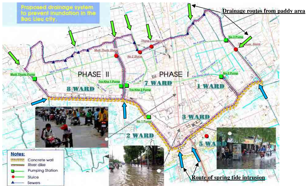
Figure 6.4.8 General Layout of Inundation Protection Plan for the Bac Lieu Center (Source; Sub-IHESV and Study Team)
