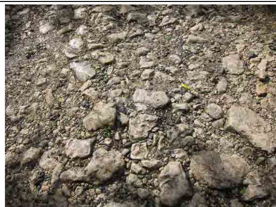
Photo 1-2 widely used Limestone pebbles for roadbed material because of its physical characteristics
