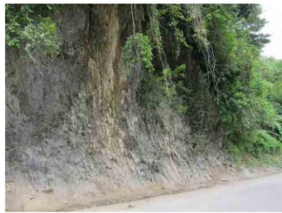
Photo 1-4 An outcrop which contributed to determine the boundary condition of limestone and older sedimentary rocks. They come in contact with conformity condition.
