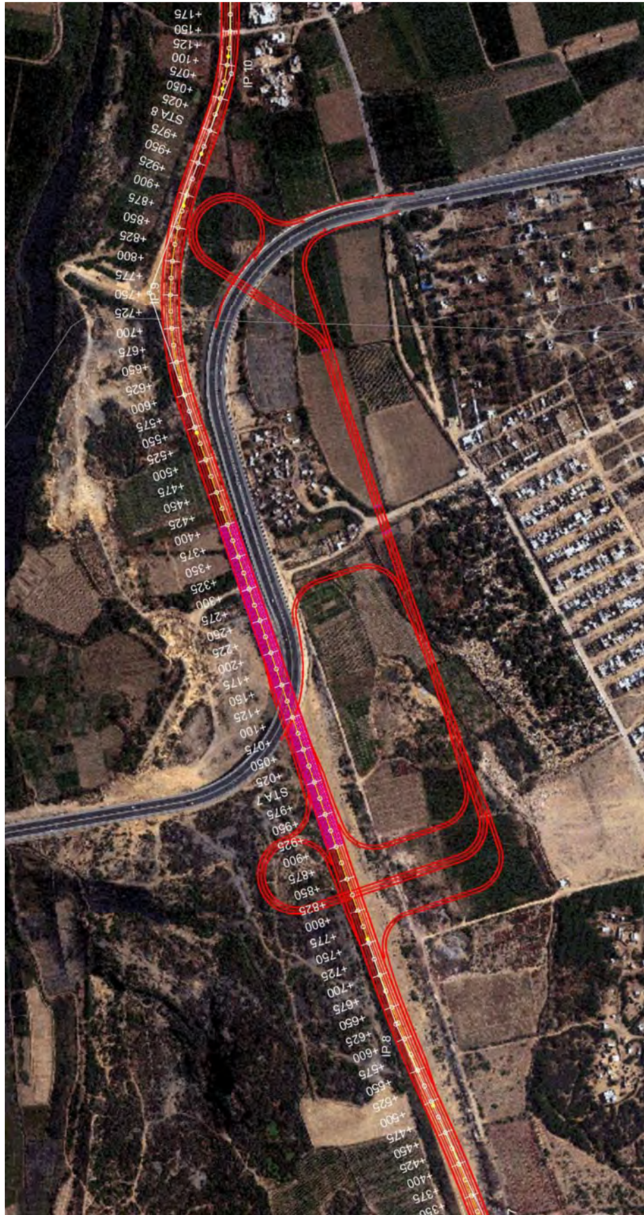
Figure 6.1.12 Ramp 2: Double Trumpet-type Interchange (Proposed Type)
