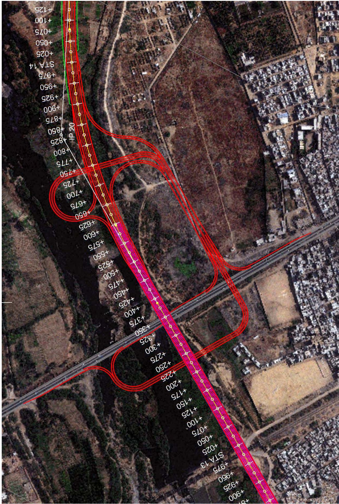
Figure 6.1.14 Ramp3: Double Trumpet-type Interchange (Proposed Type)
