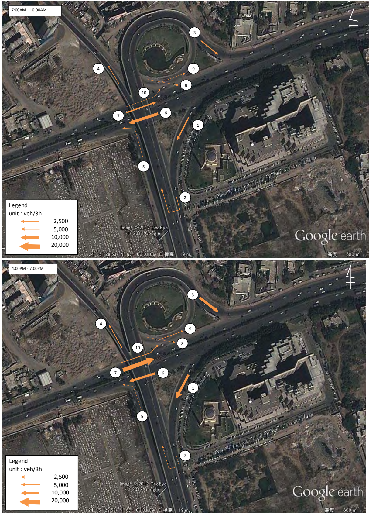
Figure 4.2.7 Traffic Flow of FTC Intersection (Morning and Evening)
