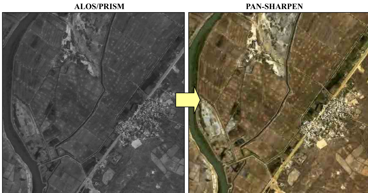
Photo 1-2 Example of pan-sharpen image (ALOS/PRISM & AVNIR-2) showing a suburb of Saint Louis in the study area
