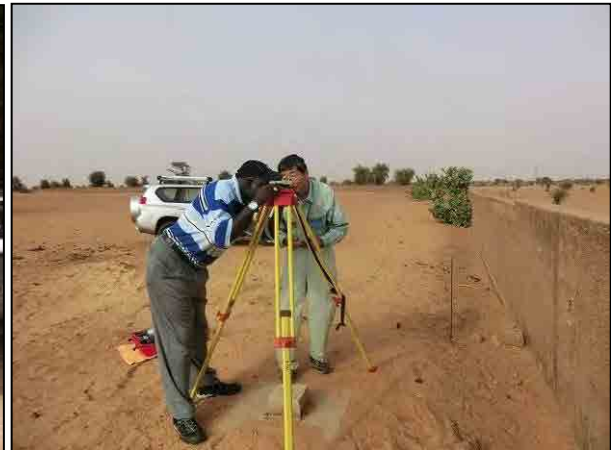
Ground control point survey - Training for centering
