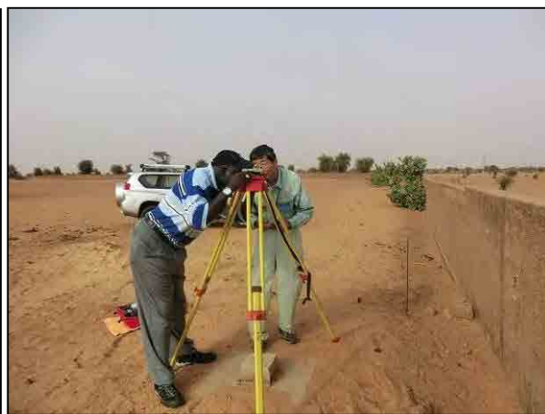
Ground control point survey – Training for centering
