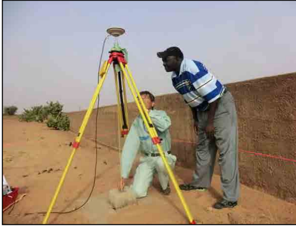
Photo 3-1 Teaching how to set up a tripod
