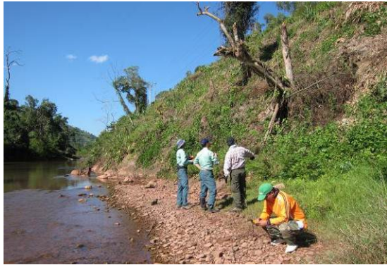
Photo 1-3 Arenite Outcrop and Sand and Gravel Sediments in the Left Abutment of Intake Site
