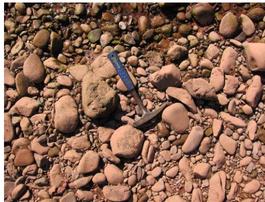
Photo 1-6 Gravel Layer Covers the River Bed Which Consists of Sand and Some Cohesive Soil
