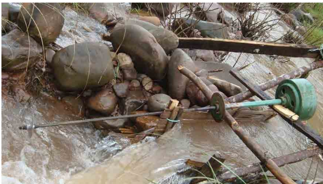
Image 4-3b, is a closer view of the main components of a Pico unit.
