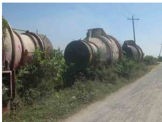
Photo-4: Former approximately 30-year-old hydropower project planed at the existing irrigation gate near the Site was canceled due to mismatch of the site condition and procured turbines which still remain at the project site.
