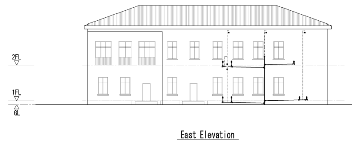
Jomi Central District Hospital / renovation Pediatric Ward Drainage pipe exterior laying elevation plan
