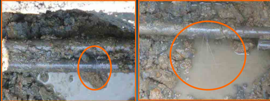
It was measurement of trace amount of water from PVC pipe leak from a needle hole
